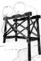
GAS and OIL RACK
