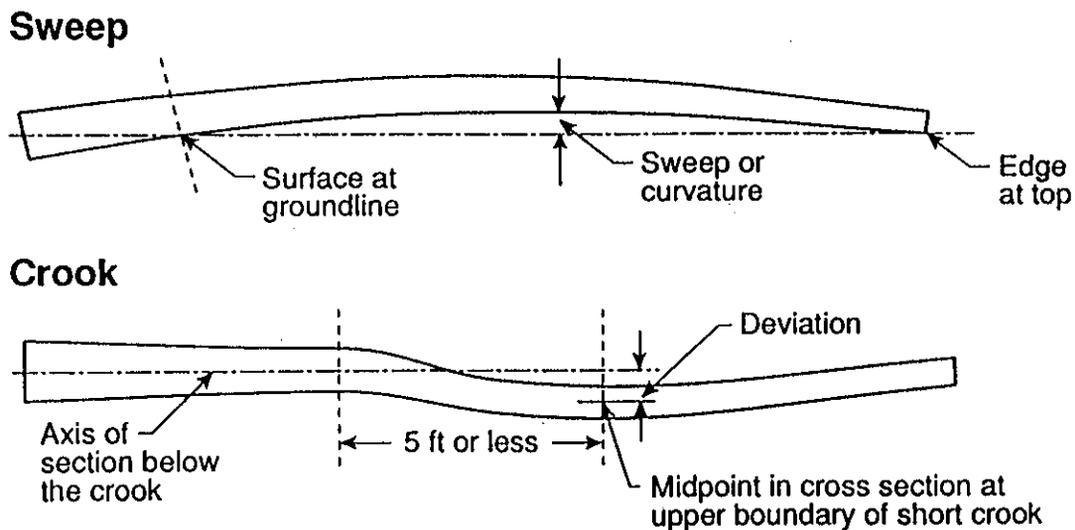
Figure 2. Pole shape limitations (1 ft - 0.3048 m).
